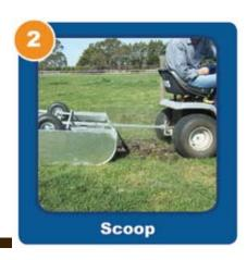
When full, take the Super Scooper off your tow vehicle then pull the pin out of the draw bar. The bar can now be swapped to the other end of the Super Scooper. It's as simple as sliding the draw bar pin and pushing the pin into place.
